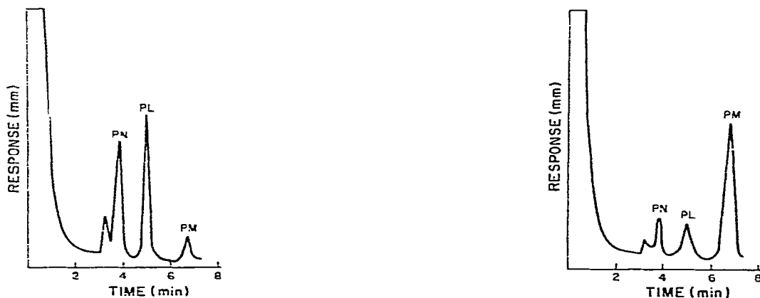
Fig. 1. Separation of B-6 standards by GC-ECD. Conditions: Microtek MT-220; column, 1.54 m \times 2 mm I.D., glass, packed with 10% SP-2100 on Supelcoport 80-100 mesh; column, 125°C, injection port, 205°C, detector, 350°C; carrier gas, nitrogen at 30 ml/min; ^{63}\text{Ni} ECD.
